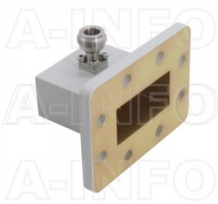
159WCAN Right Angle Rectangular Waveguide to Coaxial Adapter 4.9-7.05GHz WR159 to N Type Female
