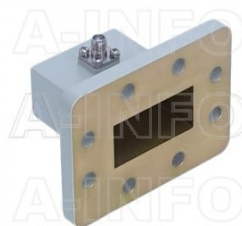
159WCAS Right Angle Rectangular Waveguide to Coaxial Adapter 4.9-7.05GHz WR159 to SMA Female
